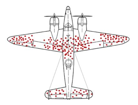
Figure 4 Location of the hits in the aircraft. McGeddon, CC BY-SA 4.0, via Wikimedia Commons. Illustration of survivorship bias, inspired by the seminal paper of Abraham Wald "A method of estimating plane vulnerability based on damage of survivors" (1943) [8]
